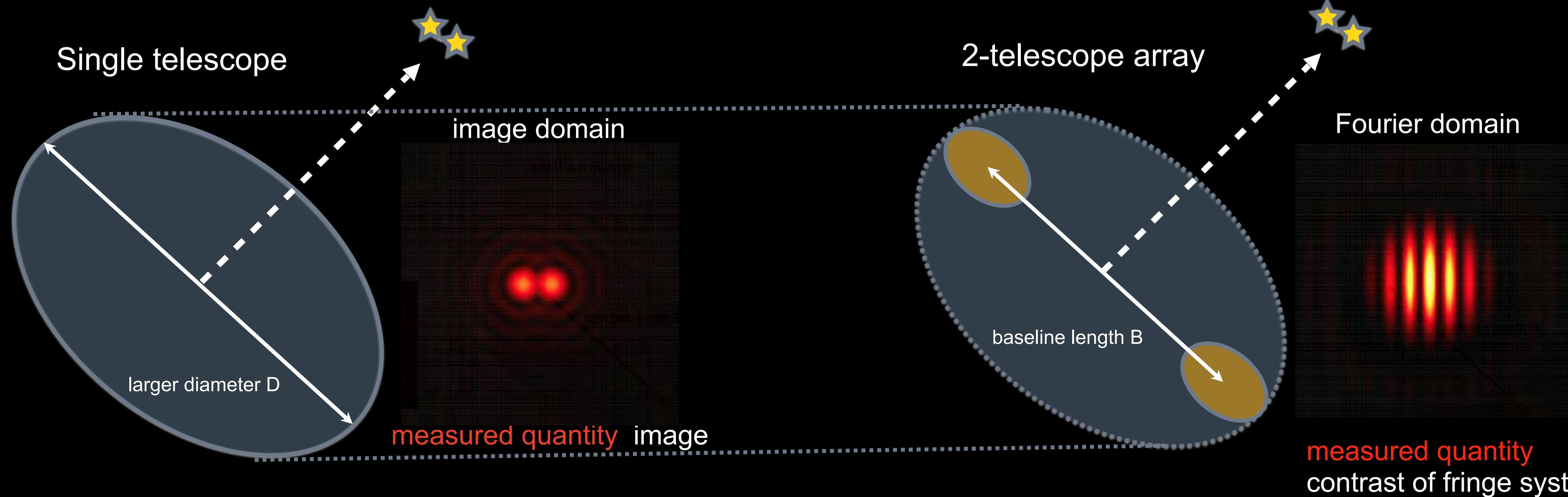
Instead of building larger telescope mirrors (which is very expensive), one can combine the light of several smaller telescopes that are separated at large distances, called baseline lengths.
